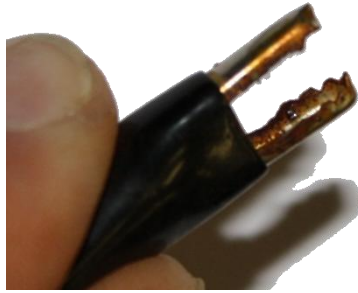
Figure 27: Corrosion of the clamps connected to the primary anodes
