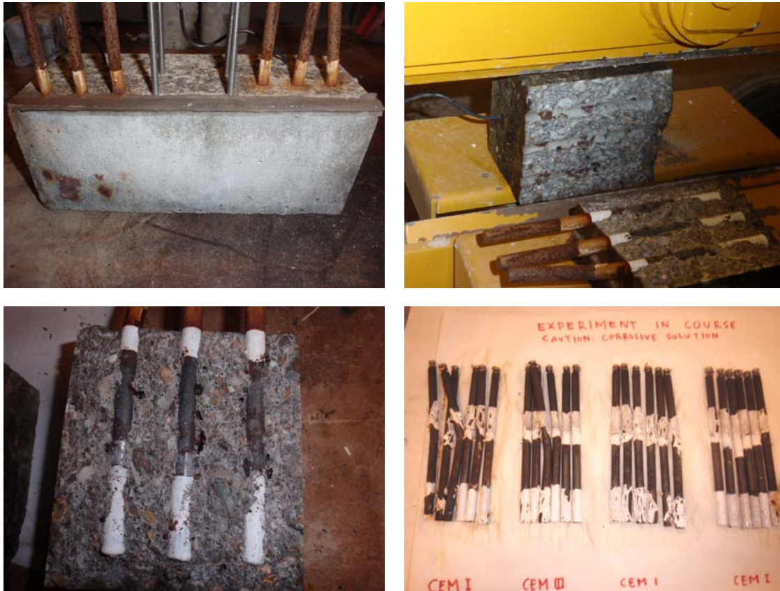
Figure 7.9 Destructive analysis of specimens after CP.
